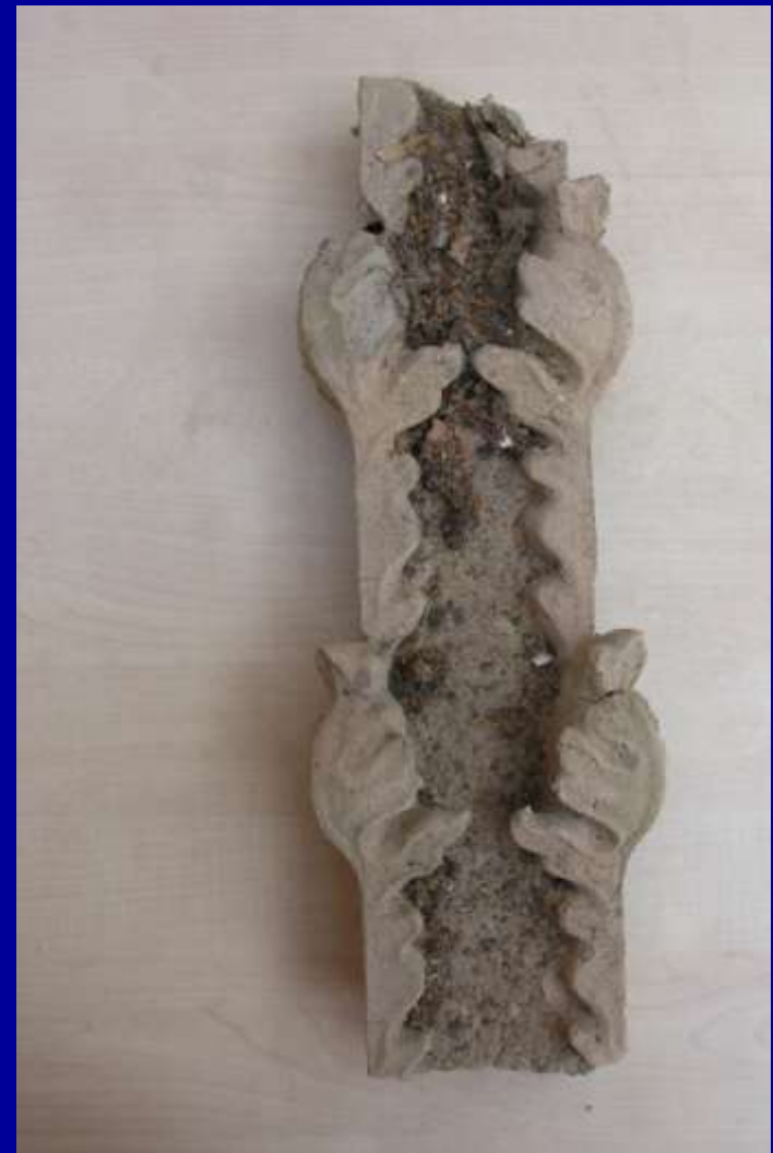
Hadlow Tower; small part of spirelet cast ( right) and complete replica for mould making.
